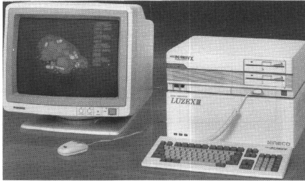
Fig. 2. An example of image analyzer, Luzex III by Nireco Cooperation.
